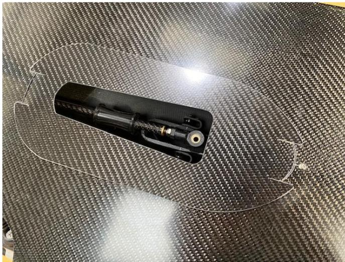
5, fit the fairing clips- push the central piece to secure, to release use a small screwdriver to push the central piece through.
