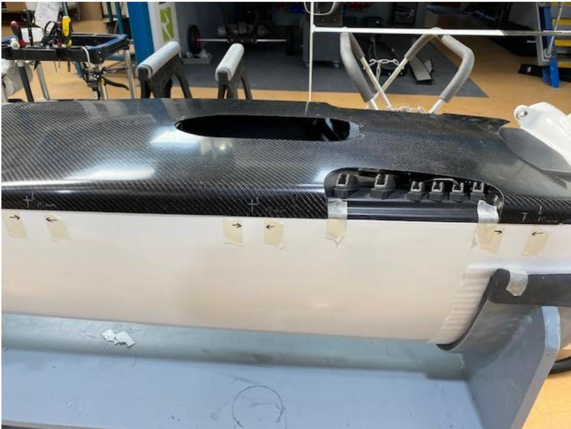
4, Reposition the fairing, mark the holes for the fairing clips
