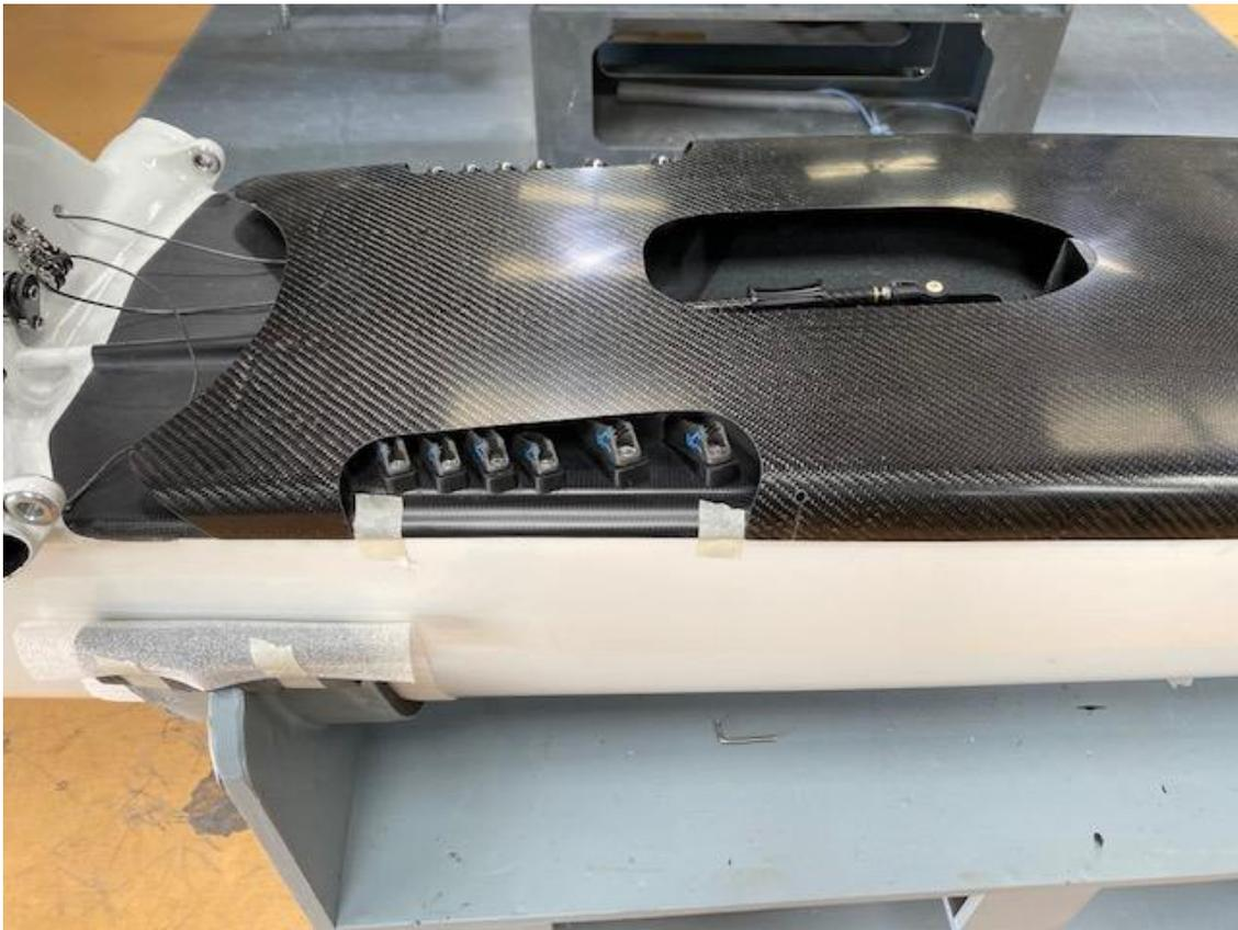
1, Dry fit the fairing, ensure it clips into the tramp track. Once happy with the position mark the cleat cut out with tape to help you re position it. Different cleats will require more of the fairing to be cut out.
