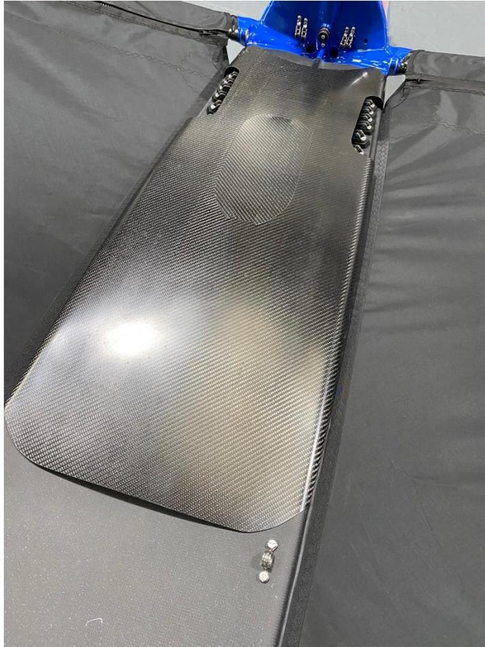
The kit comes with the smooth top plate, this can be modified or used if you are keen to modify the foil gearing set up, if not the plate with the cut out will need to be used. Fit the fairing after you have re fitted the tramps.
