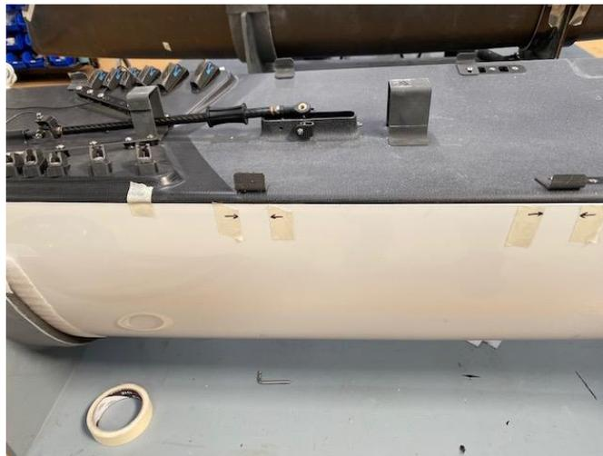
3, Transfer the bracket position to the hull below the track. Bond the brackets in place with Sikaflex 291i black, allow to cure overnight.
